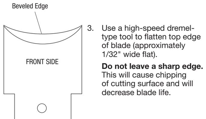
3. Use a high-speed dremel-type tool to flatten top edge of blade (approximately 1/32" wide flat).
