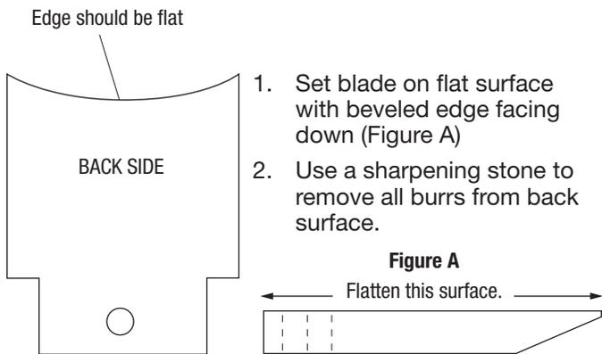
1. Set blade on flat surface with beveled edge facing down (Figure A)
